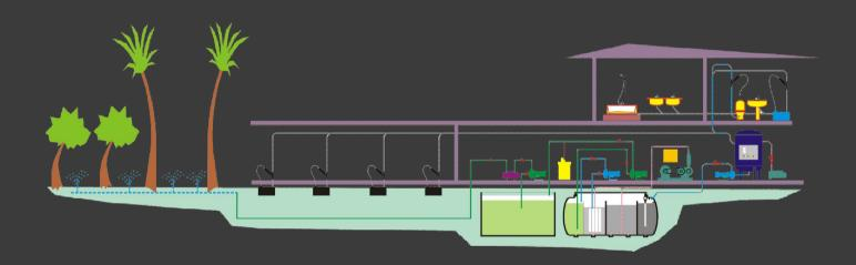
Mixed wastewater (gray & black) is collected and transferred via combined vacuum sewer line **epVAC.HIS** to the central vacuum tank, then discharged to the wastewater treatment & reuse plant, followed by double disinfection (chlorination & ultraviolet) prior to reuse in irrigation.
