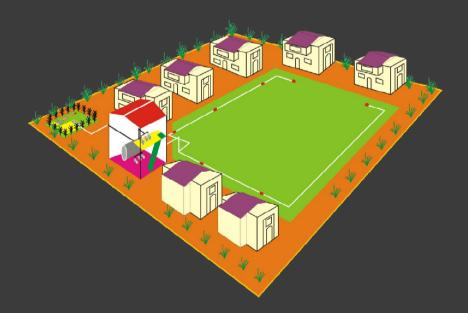
**epVAC.VSS** collects and transfers black & gray water (independently or combined), to the wastewater treatment plant **epMBR**, followed by double disinfection (chlorination & ultraviolet) prior to reuse in irrigation. Additionally prefiltration can be used for reuse in domestic non-potable water applications.
