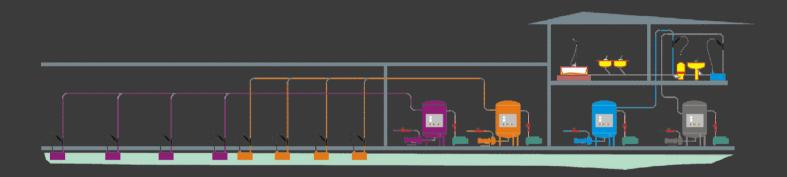
**epVAC.VSS** collects and transfers black & gray water (independently or combined), to the wastewater disposal point or to the domestic sewer network. Wastewater can be treated in **epMBR** plants followed by double disinfection (chlorination & ultraviolet) prior to reuse in irrigation. Gray water can be treated, disinfected and prefiltered prior to reuse in domestic non-potable water applications.
