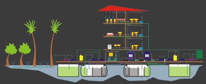
Wastewater is independently collected in gray and black water networks-**epVAC.VIS**. Black water can be treated in wastewater treatment and reuse plant epMBR followed by double disinfection (chlorination & ultraviolet) prior to reuse, then reused for irrigation Gray water can be treated in gray water epMBR plant, double disinfected (chlorination & ultraviolet) & ultrafiltered prior to reuse in domestic non-potable water applications.
