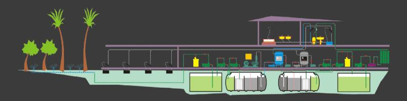
Wastewater is independently collected in gray and black water networks-**epVAC.HIS** . Black water can be treated in wastewater treatment and reuse plant epMBR followed by double disinfection (chlorination & ultraviolet) prior to reuse , then reused for irrigation. Gray water can be treated in gray water epMBR plant, double disinfected (chlorination & ultraviolet) and ultrafiltered prior to reuse in domestic non-potable water applications.
