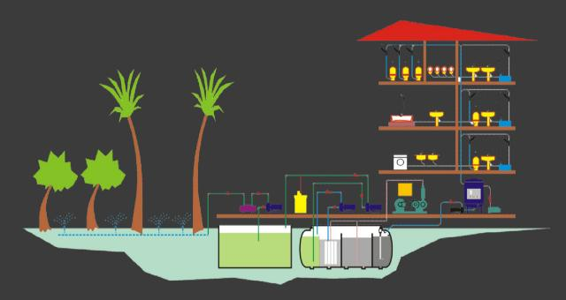
Mixed wastewater (gray & black) is collected and transferred via combined vacuum sewer line **epVAC.VIS** to the central vacuum tank, then discharged to the wastewater treatment & reuse plant, followed by double disinfection (chlorination & ultraviolet) and ultrafiltration prior to reuse in irrigation.
