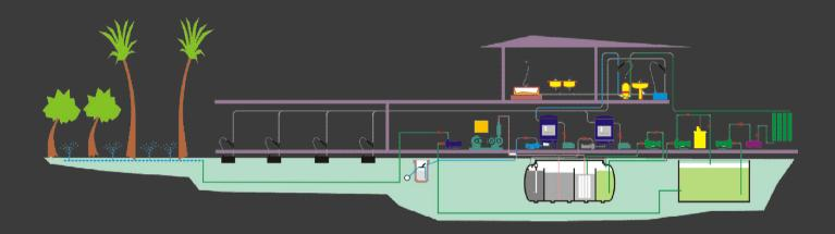
Wastewater is independently collected in gray and black water networks-**epVAC.HIS**. Black water can be discharged to the domestic sewer network while gray water can be treated in wastewater treatment and reuse plant epMBR, then reused for domestic non-potable water applications (toilet flushing, fire fighting, floor cleaning,.....etc.). **epeco** provides double disinfection (chlorination & ultraviolet) & ultrafiltration prior to reuse.
