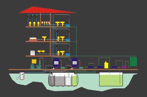
Wastewater is independently collected in gray and black water networks-epVAC.VIS . Black water can be discharged to the domestic sewer network while gray water can be treated in wastewater treatment and reuse plant epMBR, then reused for domestic nonpotable water applications (toilet flushing, fire fighting, floor cleaning,.....etc.). epeco provides double disinfection (chlorination & ultraviolet) & ultrafiltration prior to reuse.
